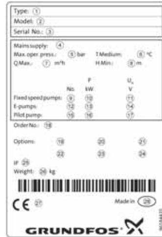
Fig. 1 Nameplate, booster system
